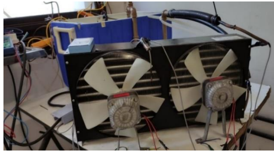
Figure 3. Cooling system of water-cooled evaporator.
