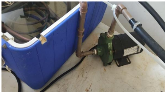
Figure 4. Water circulation system of the water-cooled evaporator.
