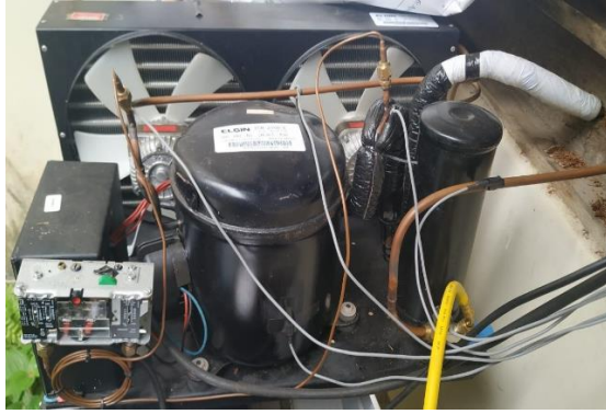
Figure 2. Condenser unit of the Chiller system test bench.
