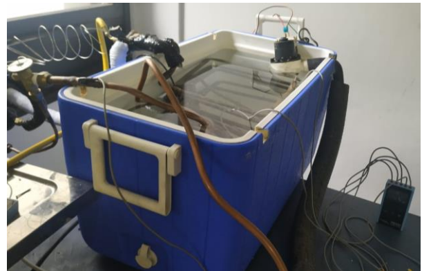
Figure 1. Evaporator unit of the Chiller system test bench.
