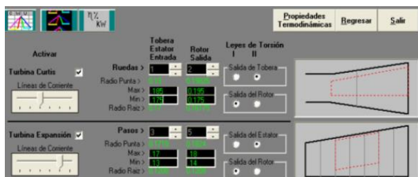
Figura 9. Panel to calculate the distribution of velocities as a function of the radius of the blade.
